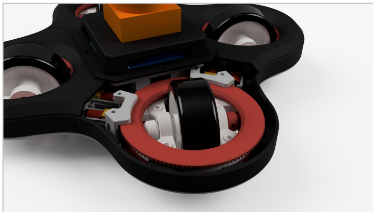
One module: two N20 motors both steer and drive the wheel
