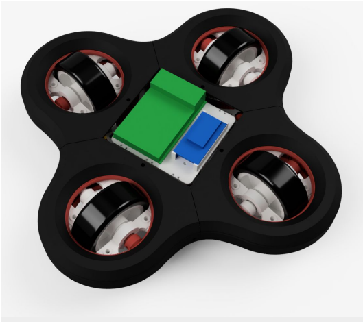
Centre bay: Raspberry Pi 5 (green) beside the ESP32 controller (blue), under a 35 mm cap
