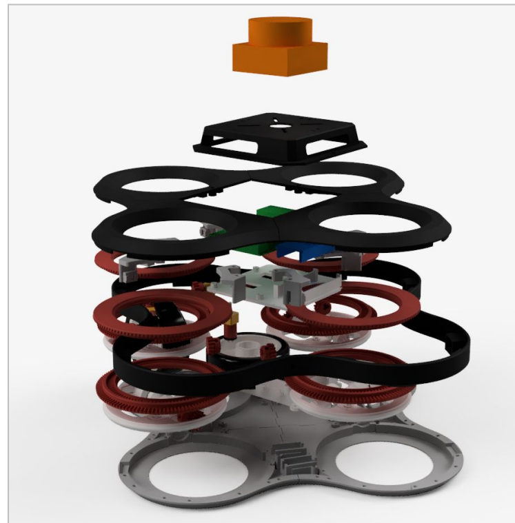
Exploded view of the printed layers
